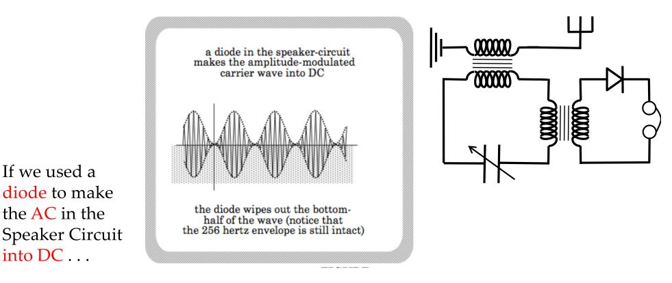
... the general trend of current will motivate the speaker to flex in and out with the average of the signal, which is to say that the speaker cone's motion will be governed by the envelope of the amplitude modulated wave, where the envelope is the same as the information wave.
