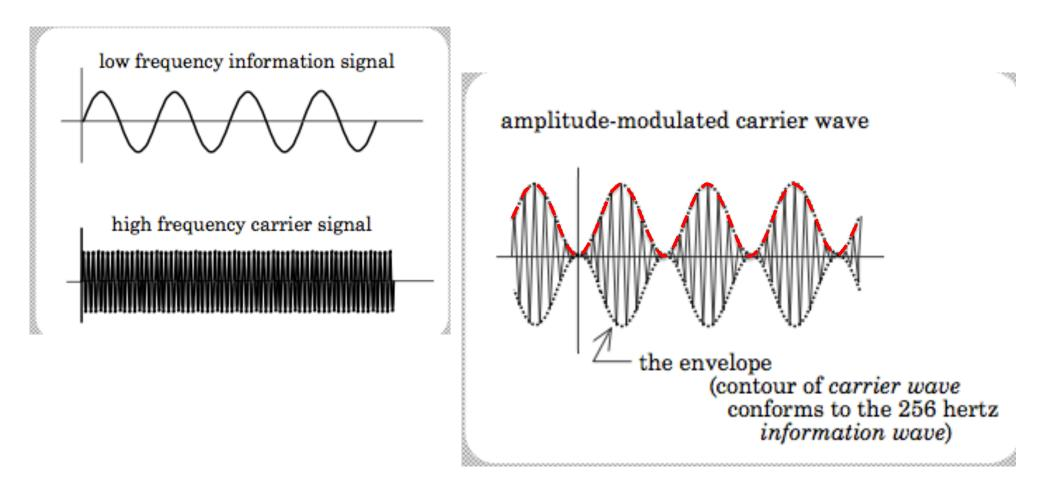
Amplitude modulation as the mode of information transfer is why these radios are called "AM" radios.
