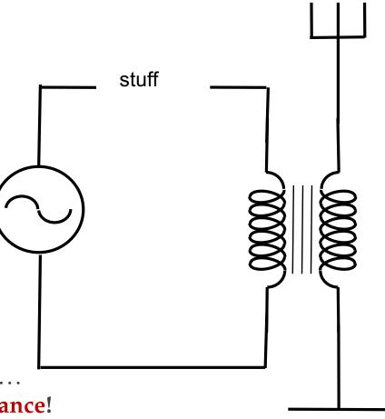
If the generator's AC is below 500,000 hz, there will be enough time for the fields to collapse back down on themselves before the new fields are set up in the region around the antenna.
